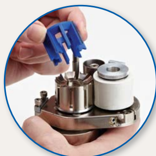
Remove used blade cartridge
